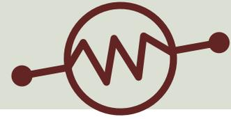
A thermistor is an electronic component that changes resistance to temperature - so-called Resistance Temperature Detectors (RTD). It is often used as a temperature sensor.
