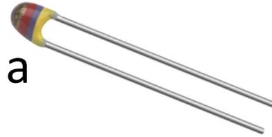
Our Thermistor is a so-called NTC (Negative Temperature Coefficient). In a NTC Thermistor, resistance decreases as the temperature rises.
